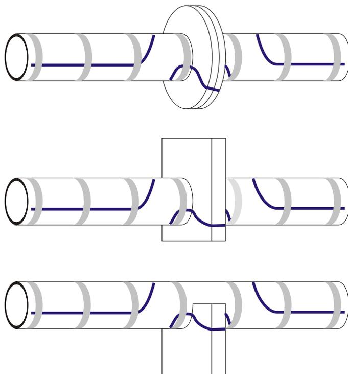
Examples of heating cable fitted on a pipe flange, suspended pipe bearers and ground supports
