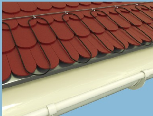
Example of heated roof edge
