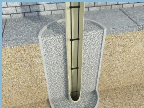
Installation of heating cable below the ground level
